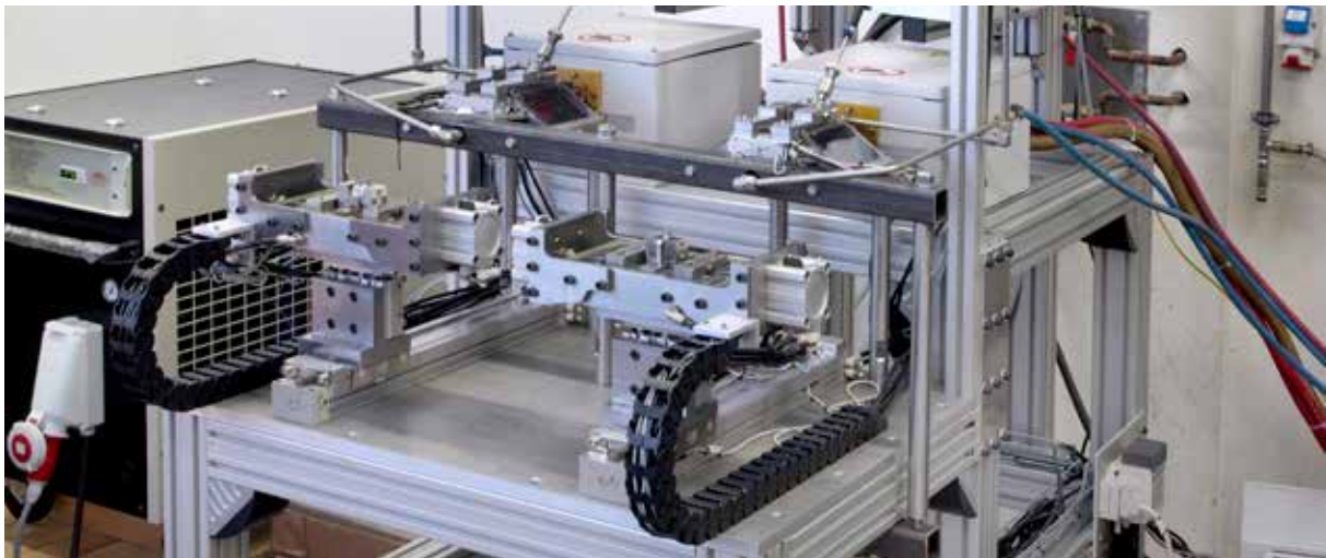
An example of a custom-designed and integrated brazing solution from EFD Induction. This particular flux-free system features two protective atmosphere brazing chambers.
