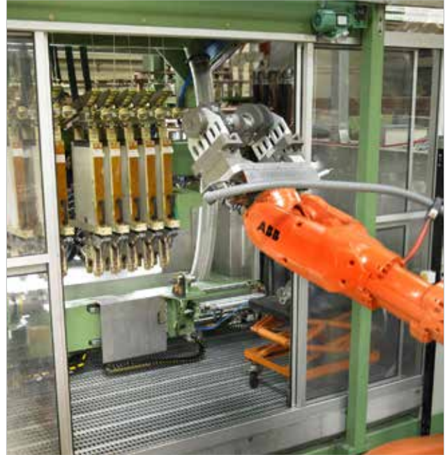
The HardLine CIHM-R hardens automotive and off-road crankshafts of any pattern up to a maximum length of 600mm.
