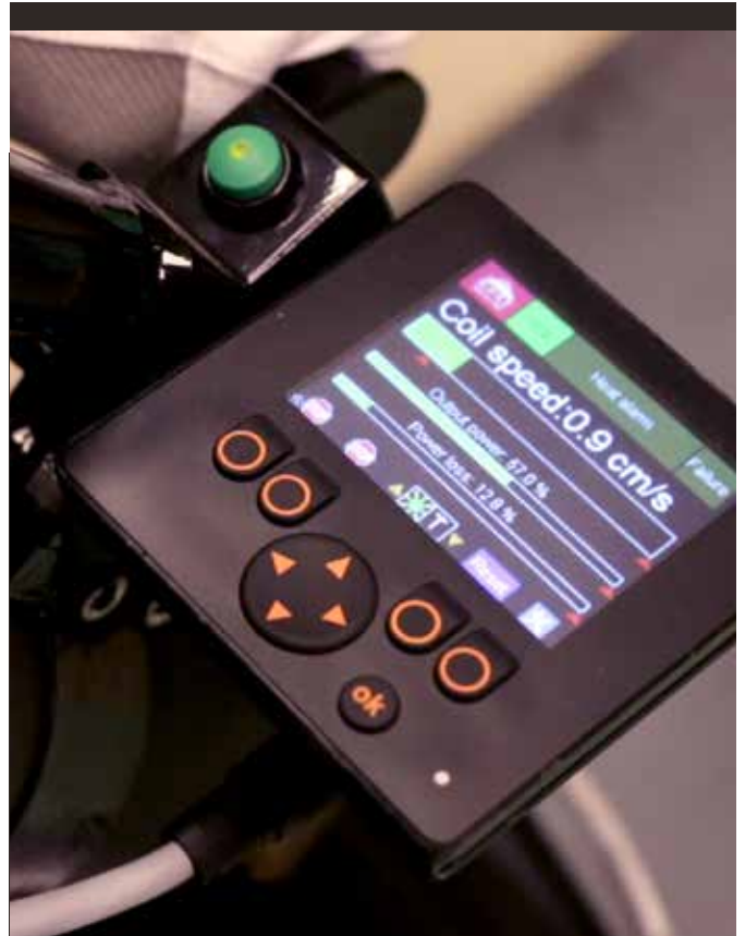
Easy-to-understand graphics Power level and heating cycle duration is automatically adjusted.
