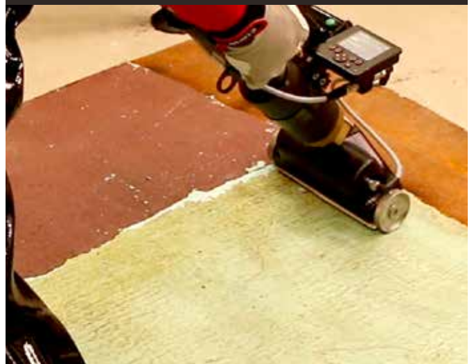
i-Scan control The scanning device responds to variations in traversing speed and the thickness of the coating.
