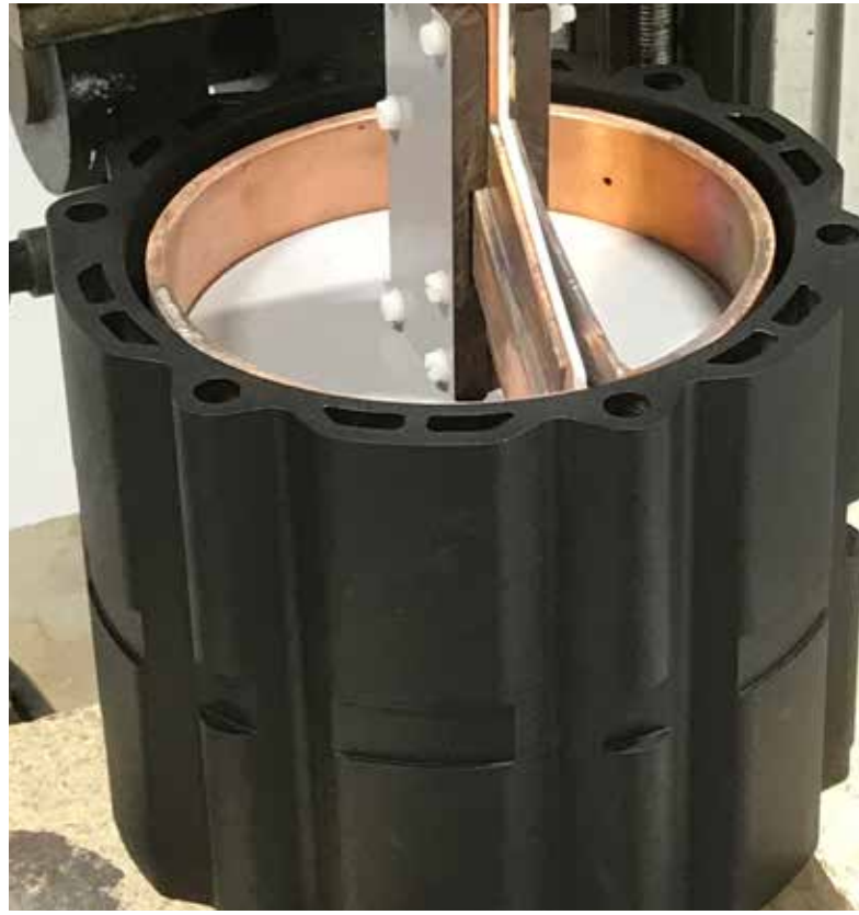
Manual solution for shrink-fitting of motor house.
