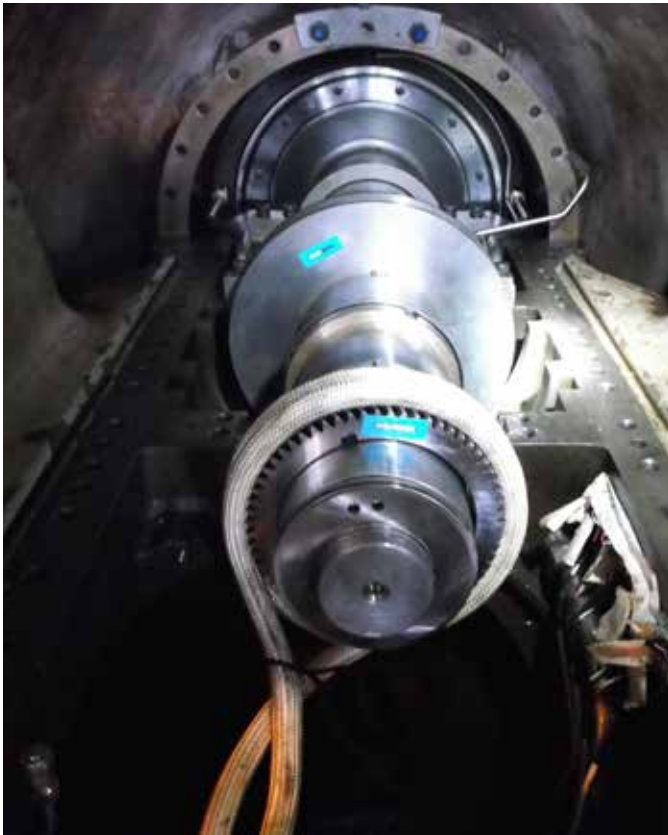
Flexible heating cables are ideal for shrink-fitting of bearings and retaining rings.
