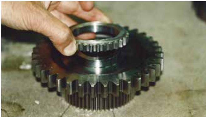
More and more automotive sub-contractors are opting for induction to shrink-fit gear wheels.
