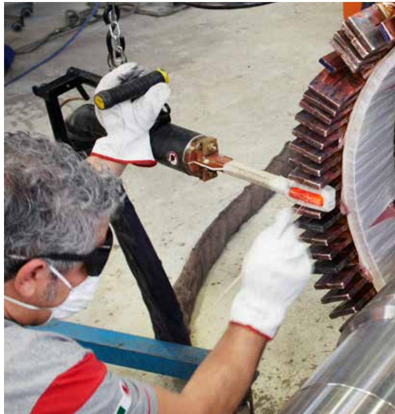
Our solutions are also ideal for induction brazing of bars, strands, rings and wires in motors, generators and transformers as well as for one-shot or segment brazing of short circuit rings.
