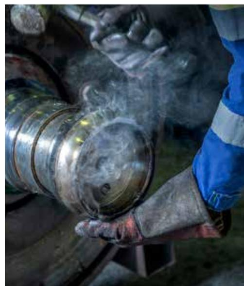
**LOCK RINGS AND BEARINGS:**The ring is heated up to a completely uniform temperature and removed while the shaft remains cold.
