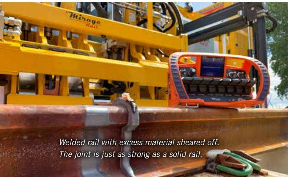
*Welded rail with excess material sheared off.
