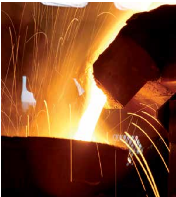
An EFD Induction single-axis tilt-pour furnace. Such systems can melt ferrous and non-ferrous metals (copper and aluminum alloys). Several models are available to suit all capacity needs. They are available with easy-to-change pre-fabricated crucibles or rammed linings.
