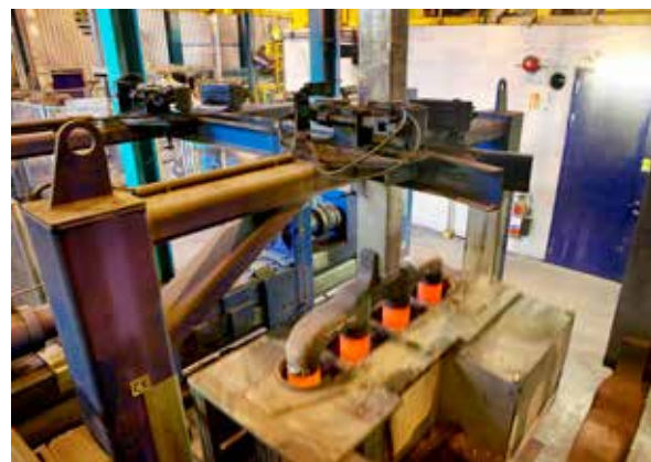
No dust, no fumes, no noise. An EFD Induction heater gets to grips with 170mm anode stubs.
