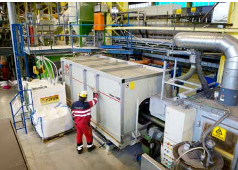
A medium-frequency EFD Induction Sinac pre-heats seamless offshore pipe prior to coating.
