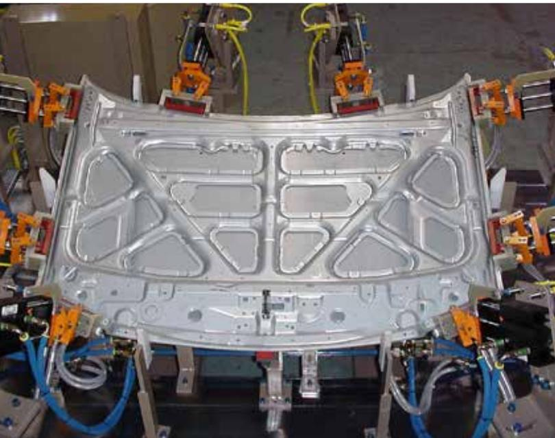
*ALUMINIUM HOOD BONDING TOOL: Note the absence of clamps, minimal nest and relatively small curing areas.*
