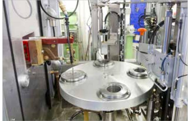
*Full automation means maximum productivity—an automatic loading magazine on a HardLine RT 550 system.*
