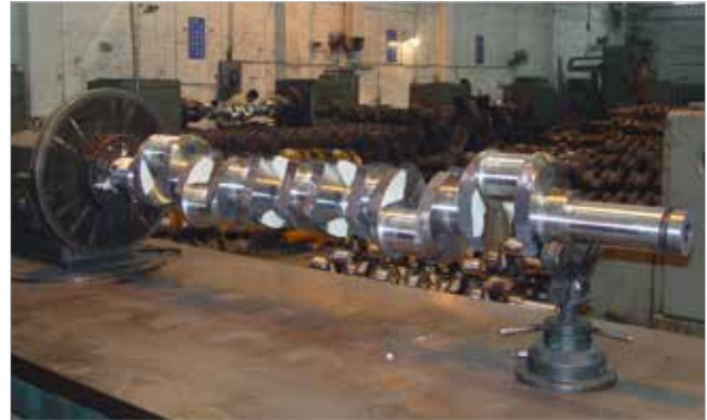
The Standard HardLine CIHM-H systems harden crankshafts of any pattern up to a maximum length of 10m.
