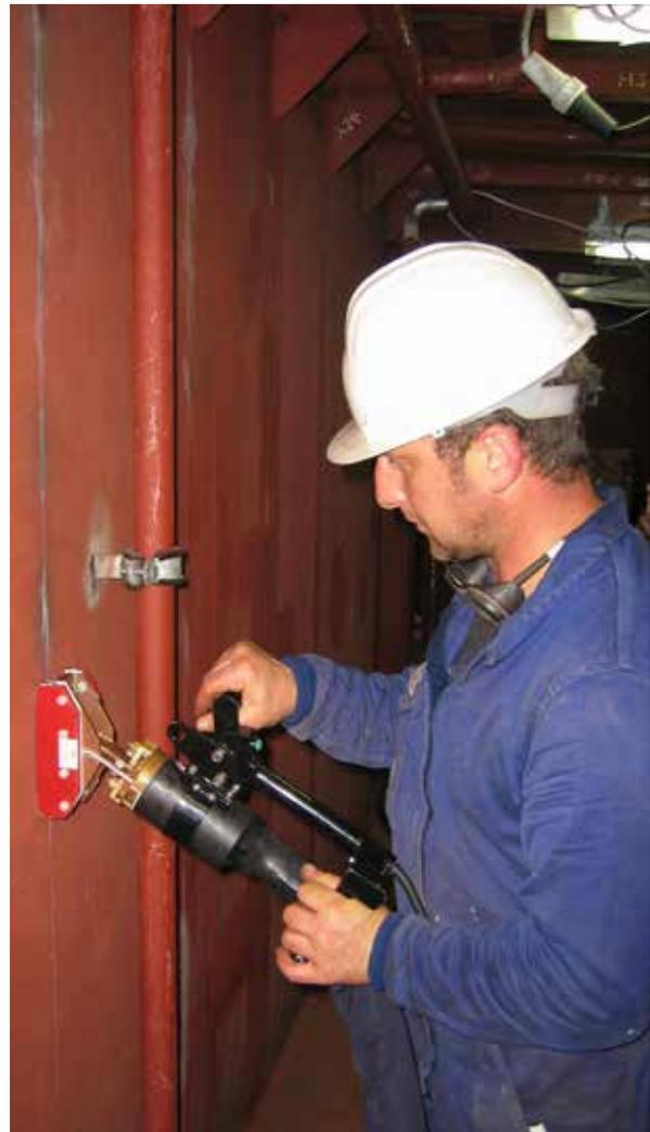
*Terac works just as well on bulkheads and other vertical structures as it does on decks. For added ergonomic comfort, the handheld transformer pictured above can be attached to a balancer and suspended from a magnet or wire rope.*
