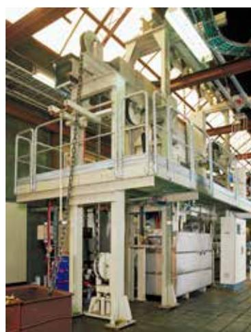
*Left, an EFD Induction engineer gives hands-on training at the start-up of a new chain heat treatment solution. Above, chain is extracted from its magazine. It will emerge hardened and tempered from the end of the line and be automatically fed to a waiting magazine or pallet.*
