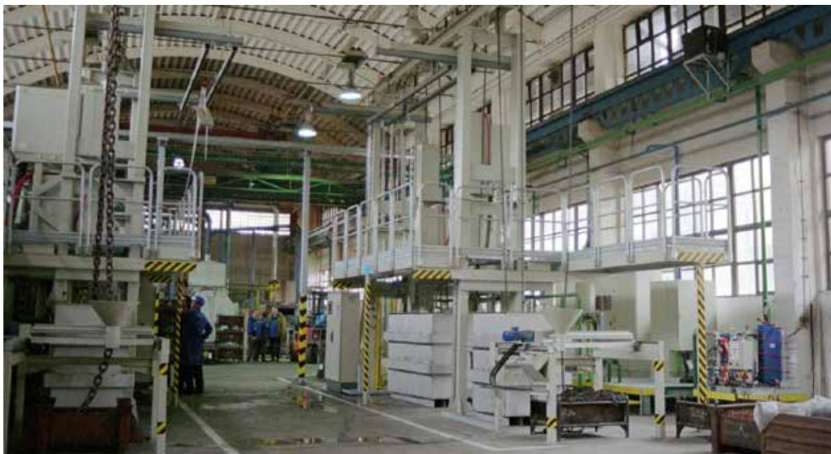
*A two-lined EFD Induction chain heat treatment solution. Our unique coil design means we can considerably reduce the height of the lines.*
