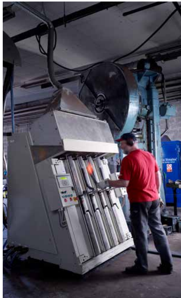
An EFD Induction CHV vertical heater. Capable of handling any type of profile, including preformed components, the CHV supports manual and robot loading.
