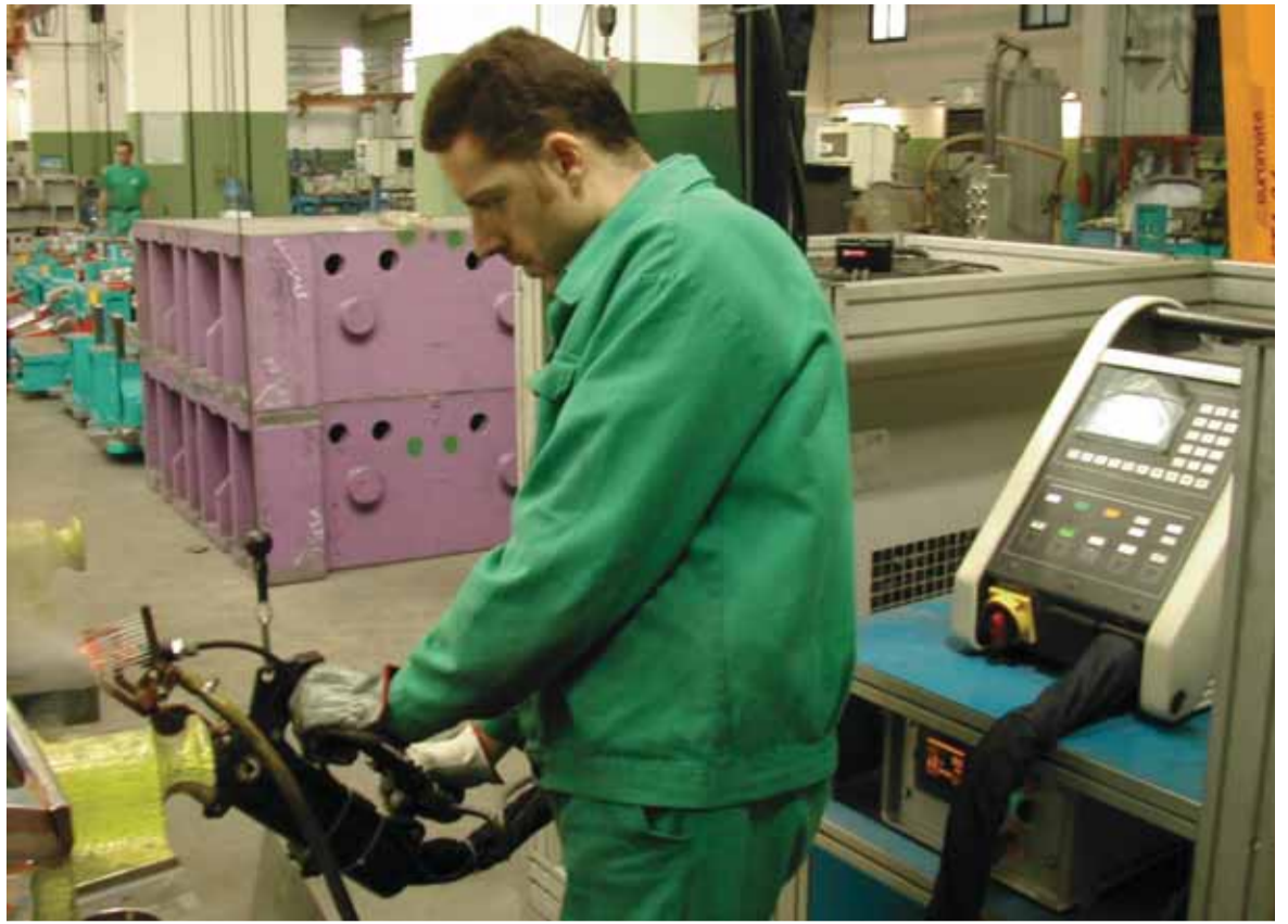
Quick, precise, repeatable. An EFD Induction solution ensures minimal deformation and a more comfortable working environment when hardening dies.
