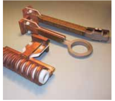
Regular maintenance of induction coils ensures high-quality production.
