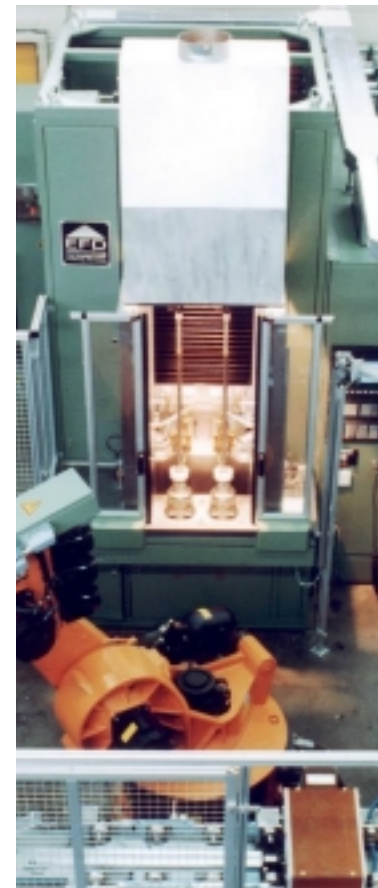
Development #1: A standard HGL machine with robot for the hardening of complete steering racks, shafts and gear parts.
