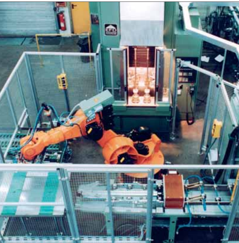
Boosting productivity: an EFD Induction HardLine vertical hardening machine with automated handling.
