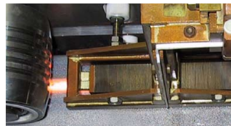
A coil heats one side of the T-beam web. A second coil simultaneously heats the other side, introducing shrinkage to compensate for weld-induced distortion.
