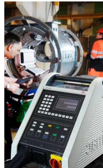
A mobile Minac being used to braze windings. The 'Twin' version boasts two independent outputs.
