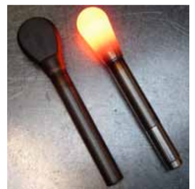
Right: a rigging component heated by induction. Left: after hot forging.
