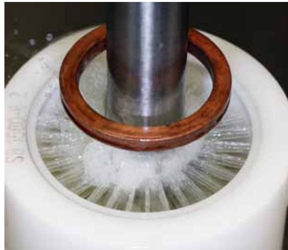
Quenching of a small gear that has been heated by the simultaneous multi-frequency method. EFD Induction specializes in customized total hardening solutions that can include workpiece loading/unloading equipment and integrated tempering.
