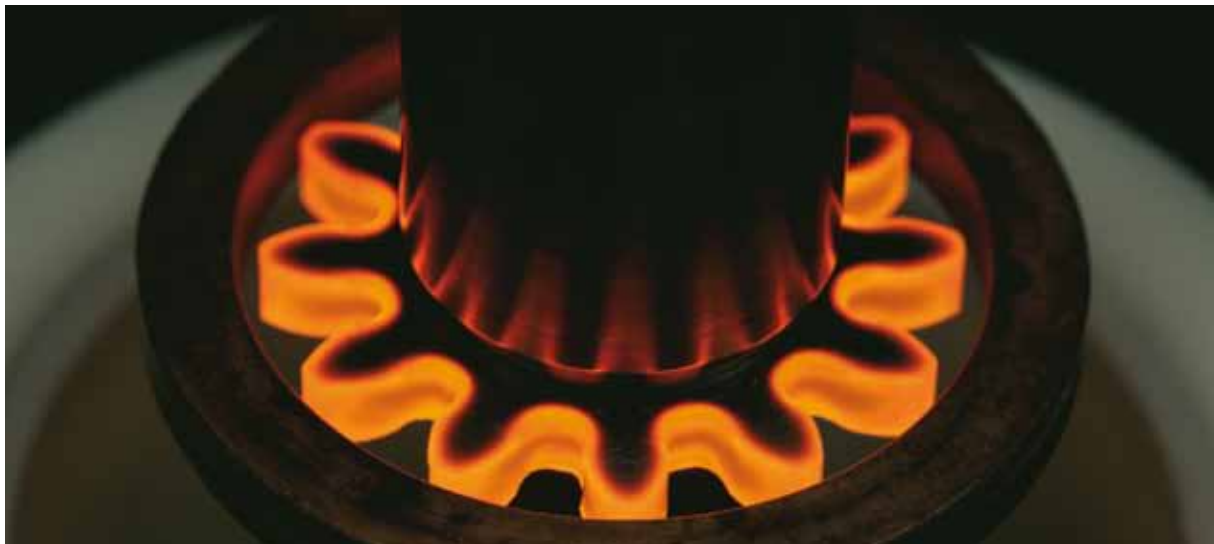
EFD Induction's patented simultaneous multi-frequency hardening in action. The process achieves true contour hardening of small gears in well under a second. Note the absence of through hardening in the teeth.
