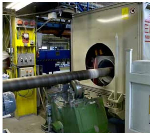
An example of induction pre-heating. The pipe is being heated prior to receiving an anti-corrosive coating.
