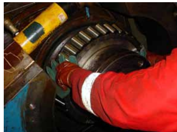
Above: Mobile induction systems perform repairs onsite—even on production platforms. Here, an operator replaces a bearing that has been heated with an EFD Induction mobile Minac system. Left: Another example of induction pre-heating, this time for pipe welding. Note the shaped copper coil that has been custom designed for this specific application.
