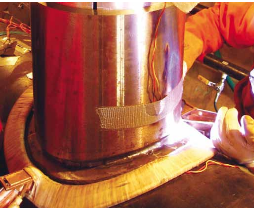
Above: Mobile induction systems perform repairs onsite—even on production platforms. Here, an operator replaces a bearing that has been heated with an EFD Induction mobile Minac system. Left: Another example of induction pre-heating, this time for pipe welding. Note the shaped copper coil that has been custom designed for this specific application.
