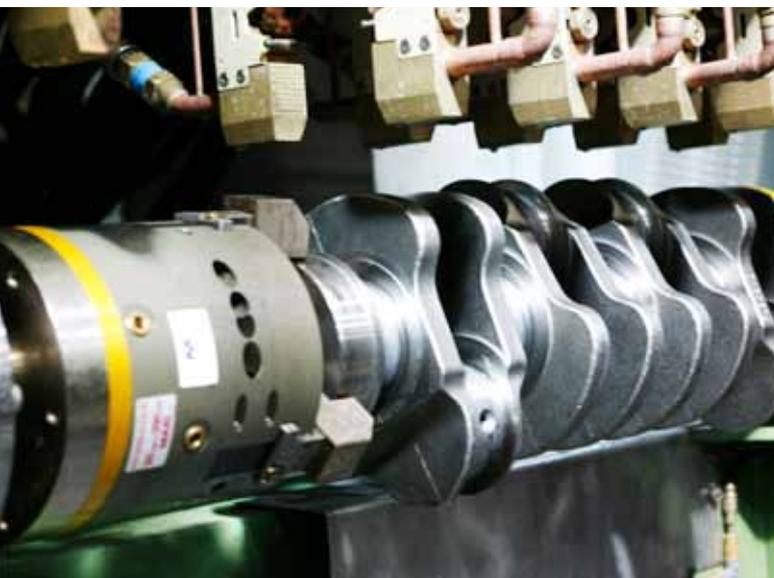
*An EFD Induction robot-type crankshaft hardening system in action. All our systems feature mechanical and control innovations that minimize Total Indicated Run-out.*
