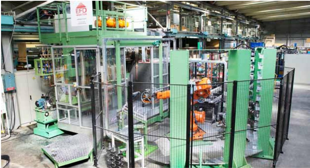
*A robot type crankshaft hardening system. Like all EFD Induction crankshaft systems, the robot type is modular. Such modular layouts are not only proven solutions, they also mean short delivery and commissioning leadtimes.*
