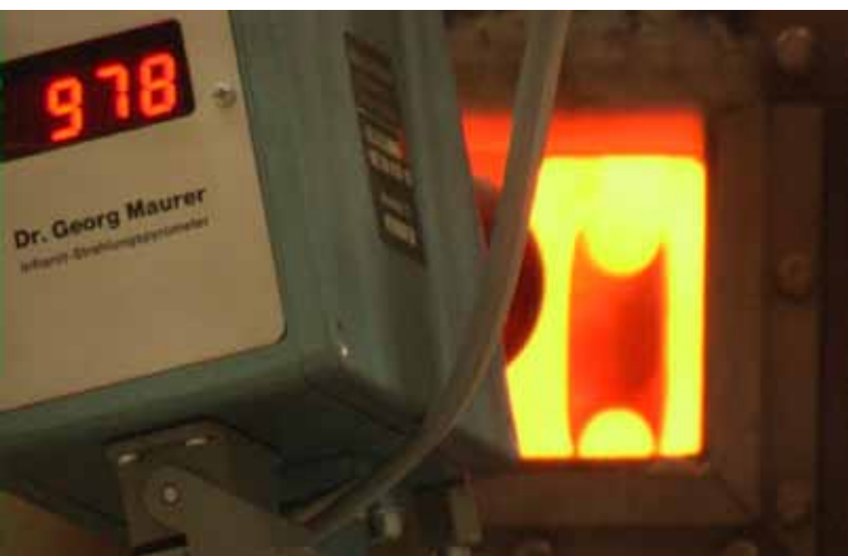
An optical heat sensor measures chain temperature. The sensor is just one of many quality assurance features available for an EFD Induction chain treatment solution.
