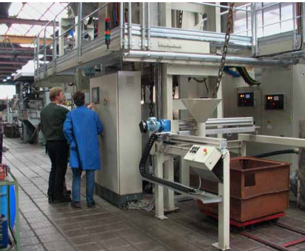
Left, an EFD Induction engineer gives hands-on training at the start-up of a new chain heat treatment solution. Above, chain is extracted from its magazine. It will emerge hardened and tempered from the end of the line and be automatically fed to a waiting magazine or pallet.
