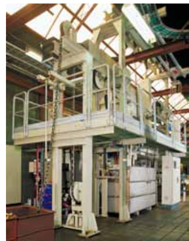
Left, an EFD Induction engineer gives hands-on training at the start-up of a new chain heat treatment solution. Above, chain is extracted from its magazine. It will emerge hardened and tempered from the end of the line and be automatically fed to a waiting magazine or pallet.
