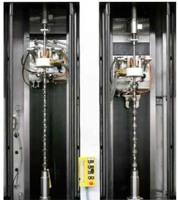
Above, a double station EFD Induction vertical hardening machine in action. Left, simultaneous quenching with polymer emulsion of two camshaft lobes.
