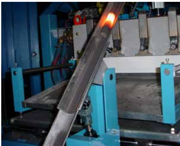
A heated workpiece being ejected from a CBB horizontal heater. The CBB ejects parts in a single location—a major benefit for operators.
