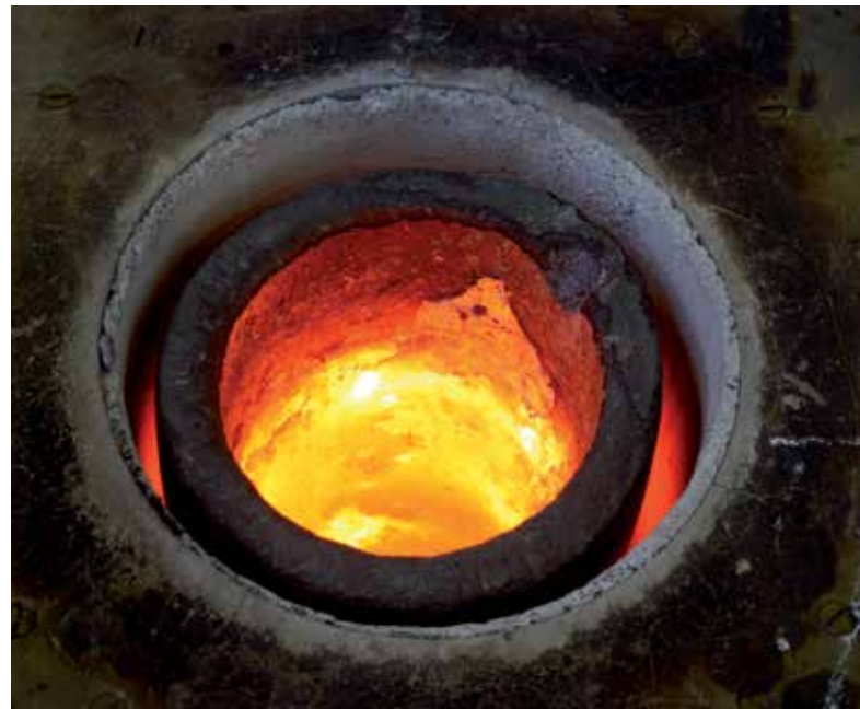
Molten brass in a moving-coil melting furnace. The pre-fabricated (clay graphite) crucible remains static during the full melting cycle. Instead, the coil moves around the crucible without touching it. Dedicated crucibles—which also act as pouring ladles—eliminate inter-alloy contamination.
