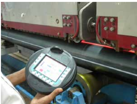
The control system helps meet the challenges posed when normalizing weld seams on the new generation of API-standard pipe.
