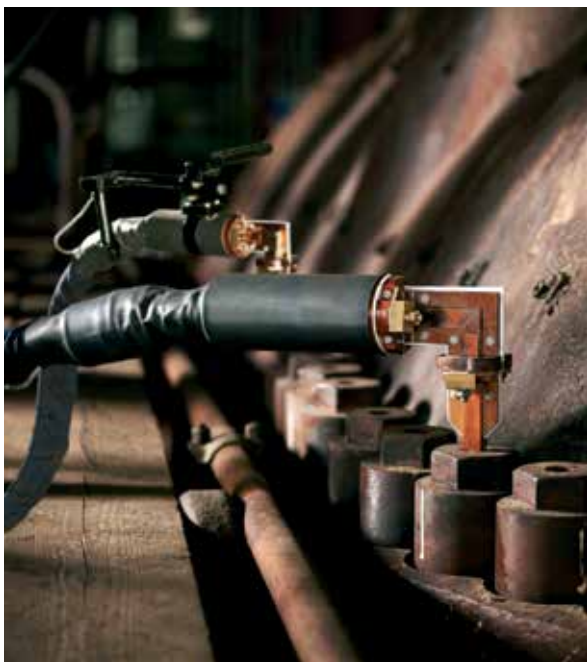
An example of shrink fitting—EFD Induction equipment removes large nuts and bolts in a fraction of the time needed by traditional gas or resistance heating.
