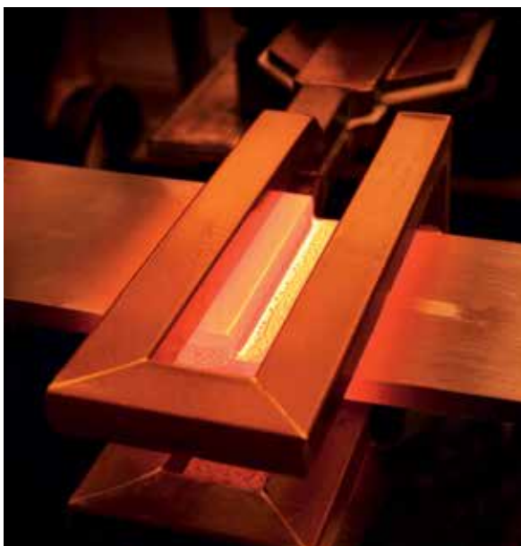
Brazing with an EFD Induction system. Note how the heating zone is fully visible, something that is practically impossible with flame brazing.
