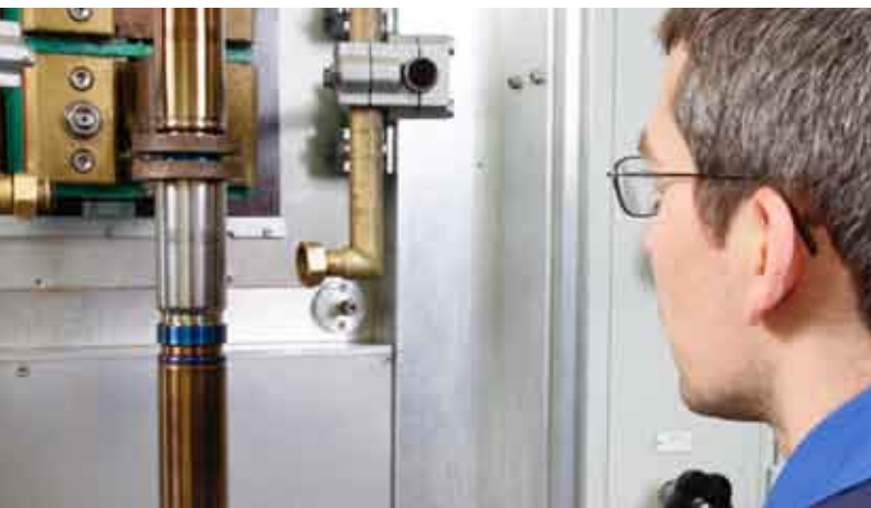
An EFD Induction vertical hardening machine in action. The chuck connection behind the workpiece lets you use the same machine for either high or medium frequency hardening.
