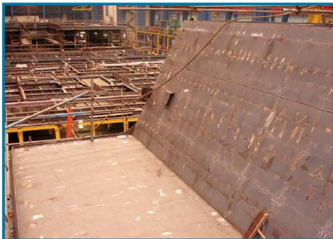
Fig. 5. Comparison between induction heated deck area and conventionally straightened angled area on right hand side.
