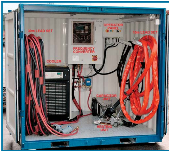
Fig. 1. Main components of the Terac heating system.
