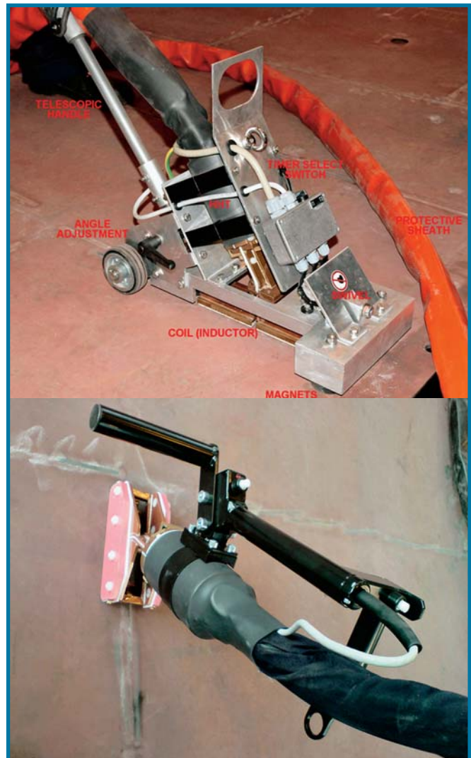
Fig. 2. Terac induction heating options: (a) Terac heating unit for straightening decks and (b) Terac heating unit for straightening vertical bulkheads.
