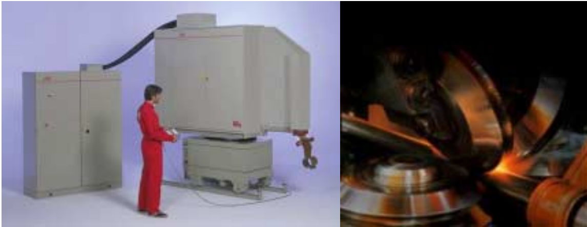
Figure 5. Longitudinal tube welding converter and the welding process
