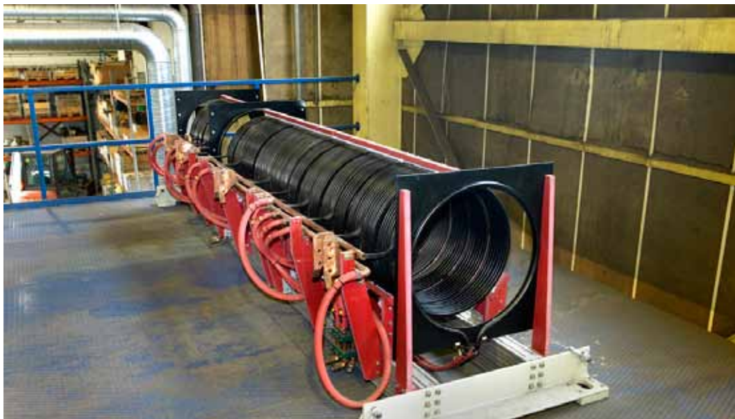
An induction coil specially designed and built for offshore industry requirements. Once heated by the coil (in red), the pipe can receive an anti-corrosion covering.
