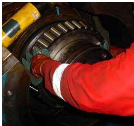
Using induction to shrink-fit components on a North Sea platform.
