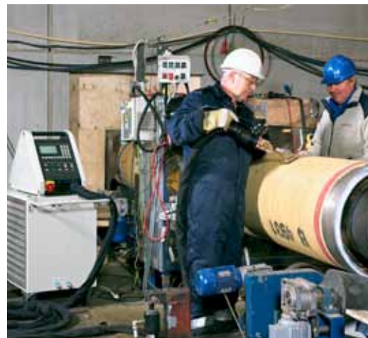
An EFD Induction mobile Minac system in action in the offshore industry. In this photo the power being applied to the workpiece is controlled by an easy-to-use handheld transformer.
